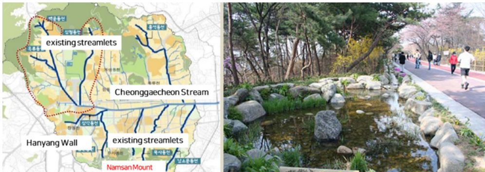
Figure 3.17 Climate-change mitigation: Restoration of abandoned streamlets, formed in pre-modern era, using a water reservoir system against heavy rainfall in Seoul's Hanyang Walled City
