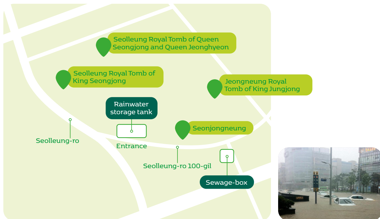
Figure 3.5 Rainwater storage(retention) tank and sewage box in Seongjongneung Royal Tomb, a World Heritage site, to mitigate flooding
