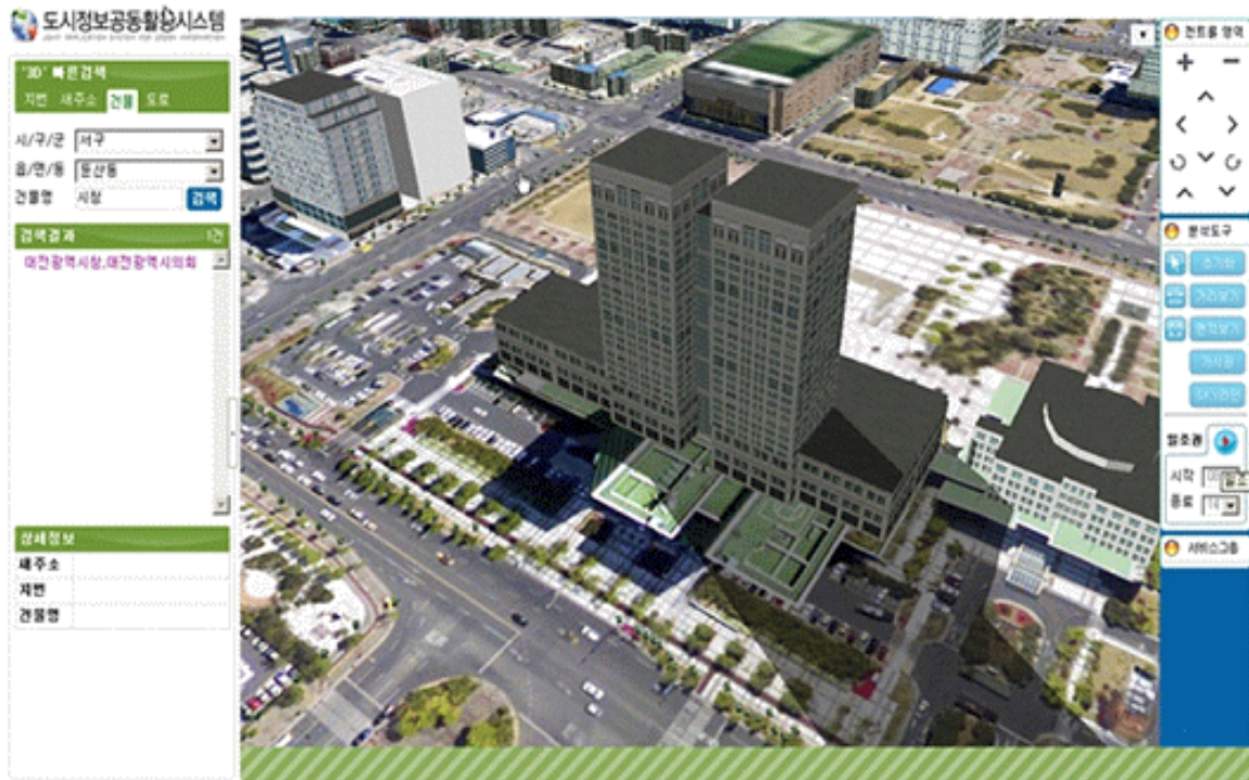
<Figure 3> The screen of analysis of right to sunshine in the 3 dimensional spatial information system
